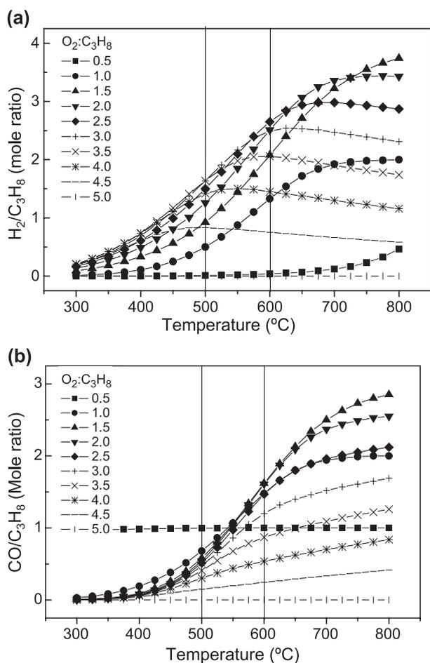
Fig. 6. Equilibrium (a)  $H_2$  and (b)  $CO$  concentrations for a range of oxygen to propane ratios as functions of temperature, assuming no carbon deposition.
