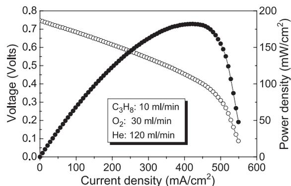
Fig. 9. Typical  $I$ - $V$  and  $I$ - $P$  characteristics for an Ni+SDC|SDC|SSC+SDC fuel cell operated at 525 °C ( $T_{\text{anode}} \sim 650$  °C) in single chamber configuration; propane, oxygen and helium flow rates of 10, 30 and 120 ml/min [STP], respectively (cell-02).
