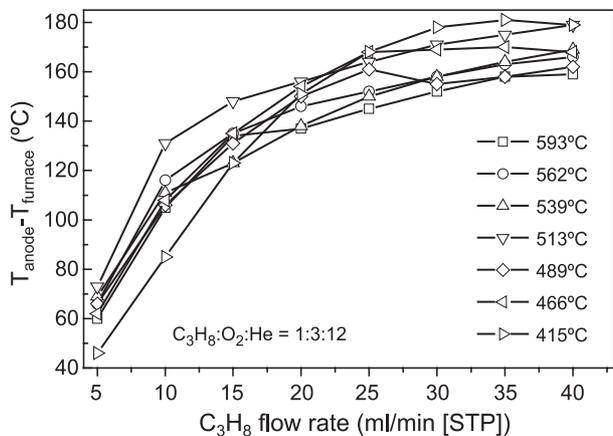
Fig. 11. The influence of propane flow rate on the rise in fuel cell temperature for the selected furnace temperatures indicated (cell-03). Overall gas composition held fixed as indicated.
