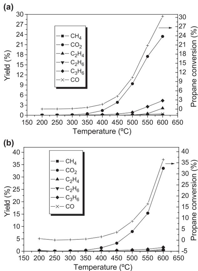
Fig. 3. Catalytic activity of SSC for propane oxidation, SSC pre-calcined at 900 °C for 5 h, 0.2 g, C<sub>3</sub>H<sub>8</sub> flow rate of 1 ml/min [STP], helium flow rate of 200 ml/min [STP], (a) C<sub>3</sub>H<sub>8</sub>/O<sub>2</sub>=1:1.5, and (b) C<sub>3</sub>H<sub>8</sub>/O<sub>2</sub>=1:3.
