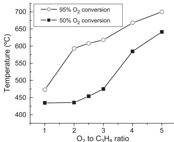
Fig. 5. The temperature at which selected levels of oxygen conversion were attained over an anode-supported half-cell (calcined at 1350 °C) as a function of the oxygen to propane ratio; propane feed rate fixed at 10 ml/min [STP], oxygen to helium ratio fixed at 1:4. The sample temperature is 80–120 °C higher than that of the furnace.
