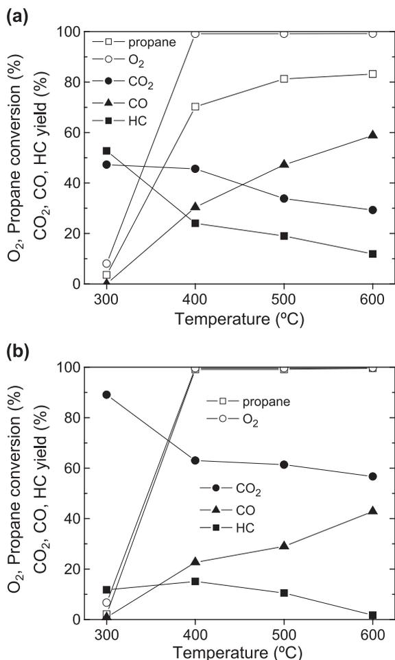
Fig. 4. Catalytic activity of Ni+SDC (0.05 g, calcined at 600 °C) towards propane partial oxidation,  $C_3H_8$  flow rate of 2 ml/min [STP], (a)  $C_3H_8/O_2/inert=1:1.6:6$ , and (b)  $C_3H_8/O_2/inert=1:3.2:12$ . Open symbols refer to conversion rates of the reactants and closed symbols to yields of the products. HC refers to all hydrocarbon species. The sample temperature is identical to that of the furnace.
