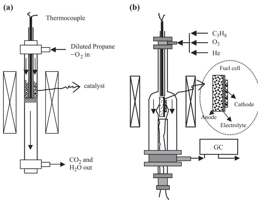
Fig. 2. Configuration of (a) the flow-through reactor for cathode and anode catalytic activity measurements, and (b) the reactor for half-cell catalytic activity and single chamber fuel cell measurements.
