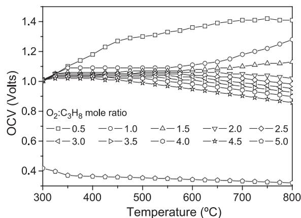
Fig. 7. Calculated OCV as function of temperature for various  $O_2/C_3H_8$  ratios as indicated, under the assumptions of equilibrium gas concentration at the anode ignoring carbon deposition and input gas composition at the cathode. Little to no carbon deposition was observed in the fuel cell experiments.
