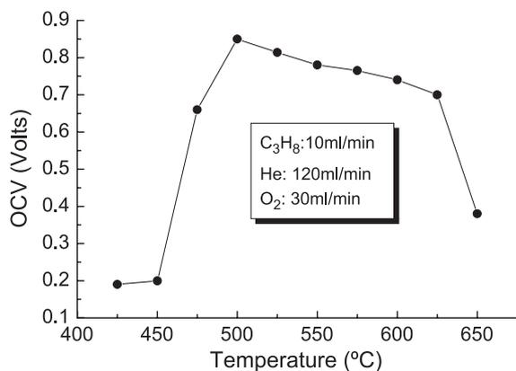
Fig. 8. Measured OCV as function of furnace set temperature (cell-01). Fuel cell anode temperature is ?.
