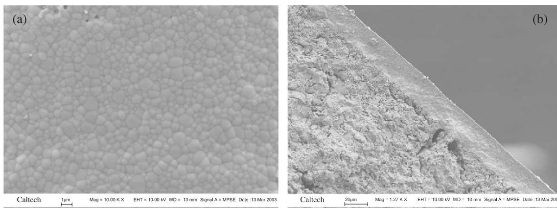
Fig. 1. SEM image of an anode–electrolyte bilayer half-cell fabricated as described in the text, (a) the SDC electrolyte surface, (b) the NiO-SDC|SDC bilayer (anode before reduction). The electrolyte has a thickness of ~20  $\mu\text{m}$ .
