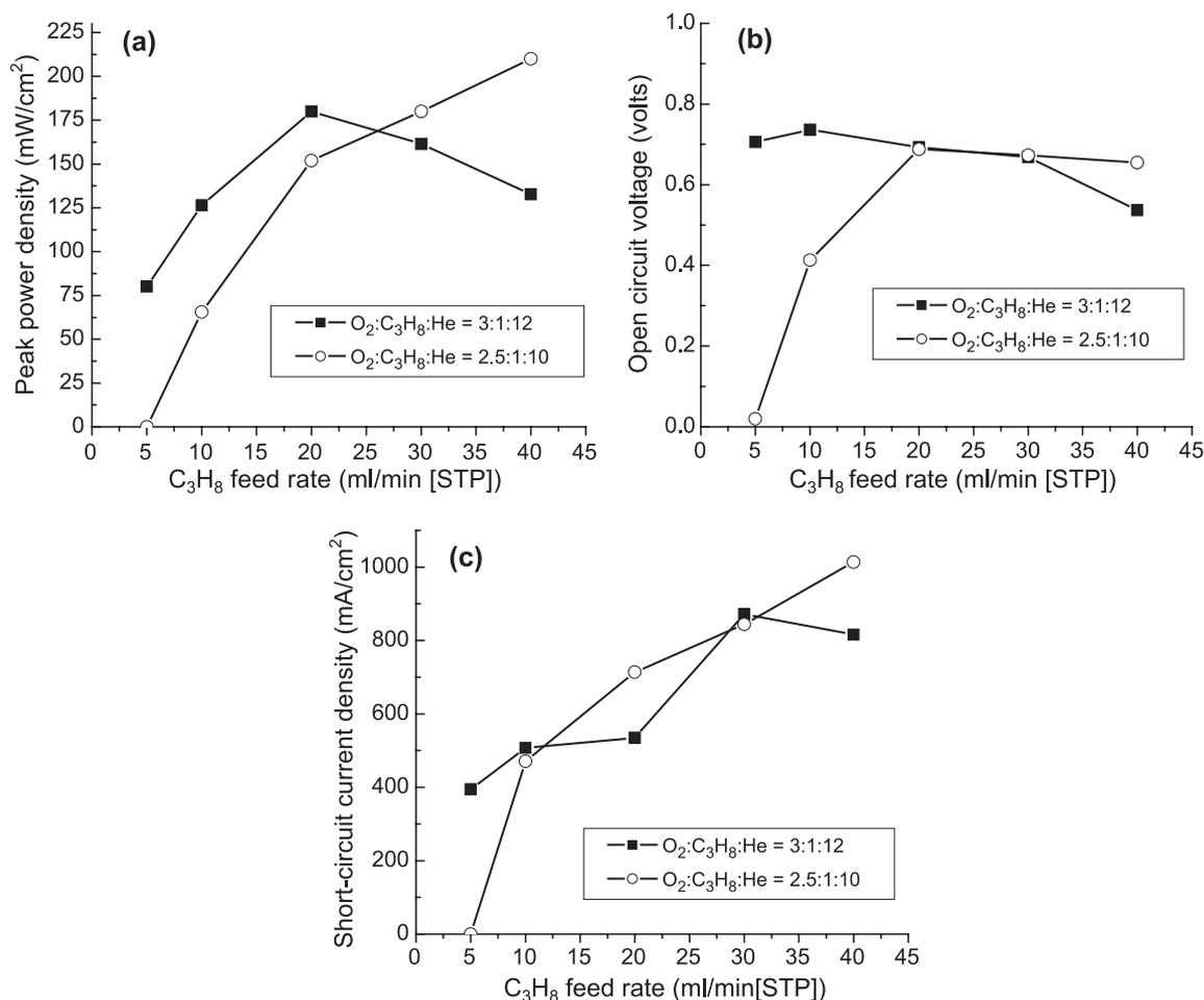
Fig. 10. The influence of propane feed rate and oxygen to propane ratio on single chamber fuel cell performance (cell-03); (a) peak power density, (b) open circuit voltage, and (c) current density at short circuit.
