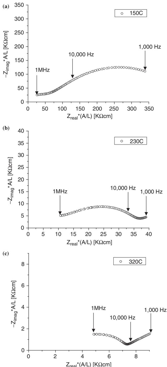
**Fig. 8.** Nyquist impedance plots for BaZr<sub>0.85</sub>Y<sub>0.15</sub>O<sub>3-δ</sub> (BYZ)-Zn4 obtained at (a) 150°C, (b) 230°C, and (c) 320°C in water-saturated nitrogen atmosphere.
