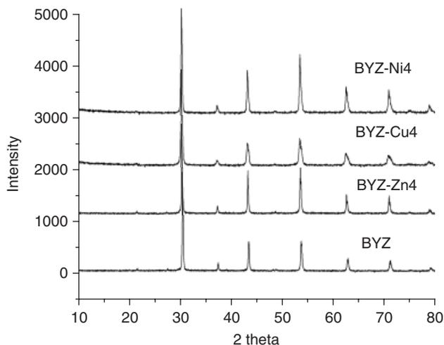
Fig. 2. X-ray powder diffraction patterns of sintered  $\text{BaZr}_{0.85}\text{Y}_{0.15}\text{O}_{3-\delta}$  (BYZ), BYZ-Zn4, BYZ-Cu4, and BYZ-Ni4.
