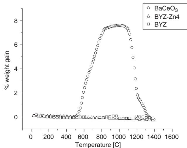
**Fig. 7.** Thermogravimetric analysis of BaZr<sub>0.85</sub>Y<sub>0.15</sub>O<sub>3-δ</sub> (BYZ)-Zn4 and BYZ as compared with BaCeO<sub>3</sub> in a CO<sub>2</sub> atmosphere.
