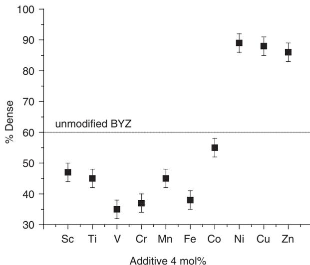
Fig. 1. Effect of transitional metal oxide additives as sintering aids for BaZr<sub>0.85</sub>Y<sub>0.15</sub>O<sub>3-δ</sub> (BYZ).
