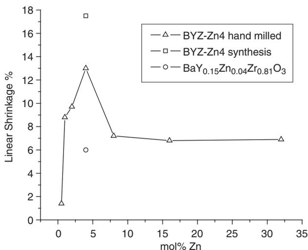
Fig. 3. Linear shrinkage of Zn modified  $\text{Ba}(\text{Zr}_{0.85}\text{Y}_{0.15})\text{O}_3$  after sintering at  $1300^\circ\text{C}$  in air (4 h) as a function of mole percentage of ZnO.  $\Delta$ , mechanical addition;  $\square$ , Zn oxide addition to BYZ nitrate solution;  $\circ$ , zinc nitrate addition to BYZ nitrate solution.
