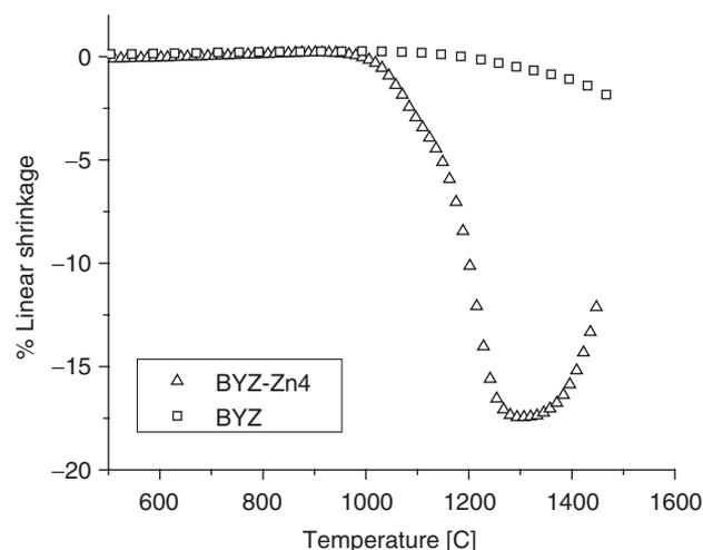
Fig. 4. Temperature dependence of linear shrinkage in  $\text{BaZr}_{0.85}\text{Y}_{0.15}\text{O}_{3-\delta}$  (BYZ) and BYZ-Zn4.
