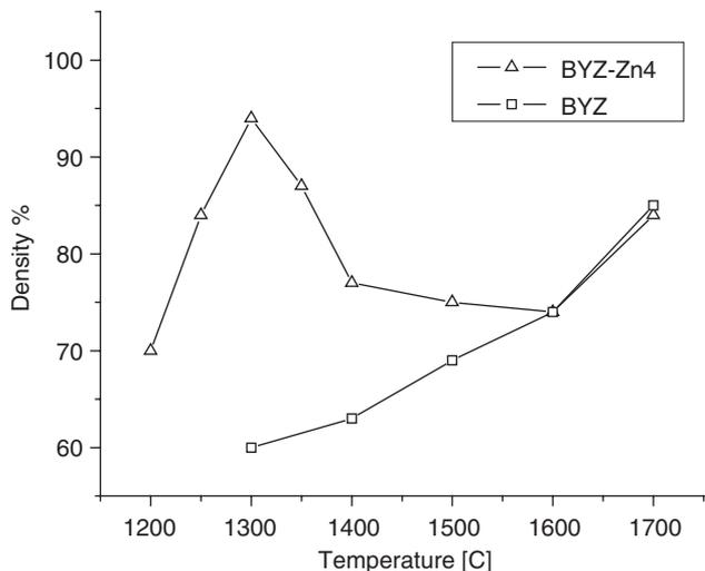
Fig. 5. Density of  $\text{BaZr}_{0.85}\text{Y}_{0.15}\text{O}_{3-\delta}$  (BYZ) and BYZ-Zn4 as a function of sintering temperature in ambient atmosphere.
