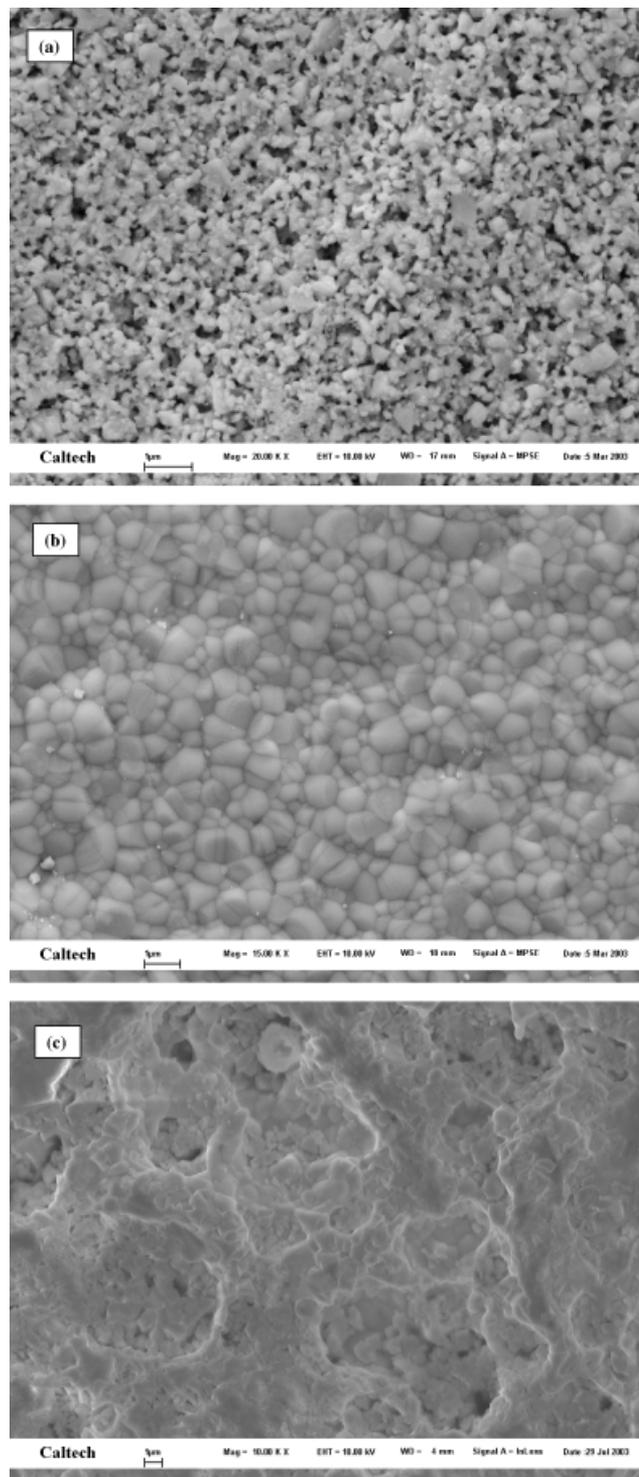
Fig. 6. SEM surface micrograph of sintered (a)  $\text{BaZr}_{0.85}\text{Y}_{0.15}\text{O}_{3-\delta}$  (BYZ) at 1300°C, (b) BYZ-Zn4 at 1300°C, and (c) BYZ-Zn4 at 1400°C.
