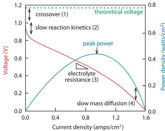
**Above left: A membrane-electrode assembly. Above right: The performance of a fuel cell is measured by a voltage-current curve that plots the drop in voltage (red) as more and more current is drawn. The blue curve is the amount of power put out by the fuel cell at a given current (or voltage). The higher the point of peak power, the better the fuel cell.**
