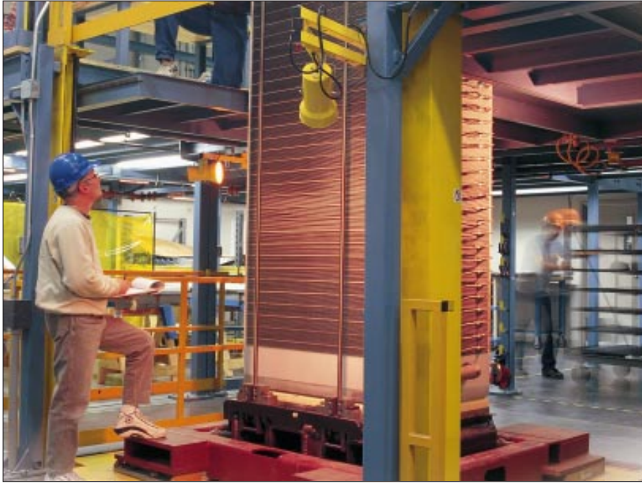
A Fuel Cell Energy (formerly Energy Research Corp) molten carbonate fuel cell
